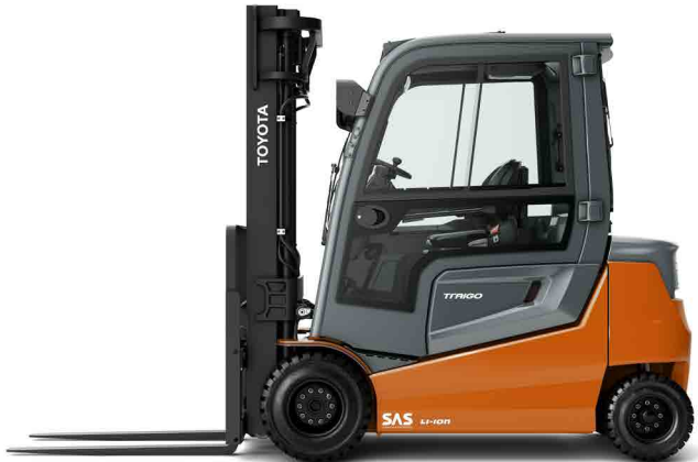
Fully floating driver compartment insulates the driver from vibration and noise for enhanced comfort and productivity.
