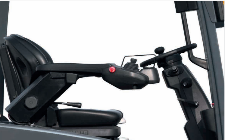
Mini-levers in the armrest offer smooth, fingertip control of lift, lower, tilt and side-shift functions.
