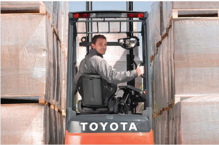
Rear-assist grip enhances reverse travel comfort and productivity by reducing operator back strain. Optional swivel seat facilitates reversing and getting in and out.
